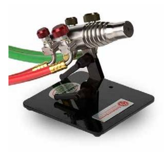
The Bethlehem Bravo Bench Burner was designed for use with gas and oxygen. Propane is the preferable gas, and is readily available from gas distributors. Be sure that your gas distributor can supply you with a pressure regulator. The regulator should be equipped with a gauge so you can see how much fuel remains in your fuel tank, and indicate the pressure you are sending to the torch.
